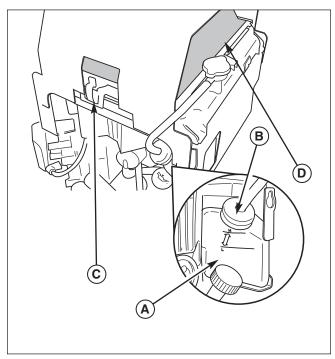
Figure 18. Radiator, Screen & Overflow Bottle
